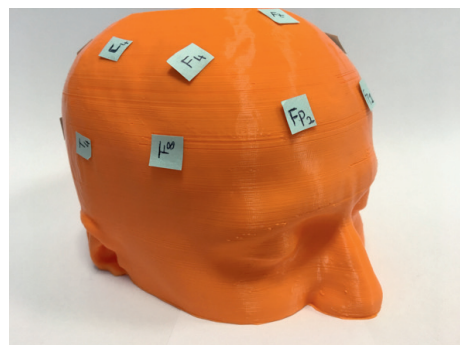
Instruction of placement of electrodes according to 10-20 system on scalp
