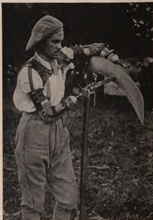
FIG. 21.—Mutilé with double forearm amputation and blind in right eye, whetting a scythe by means of the grip, Simon, and toolholder, Lauter.
